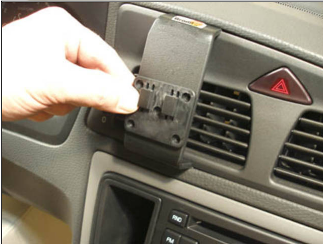
1. Place the 2 prong (Dual T) vehicle mounting plate in the desired position.
