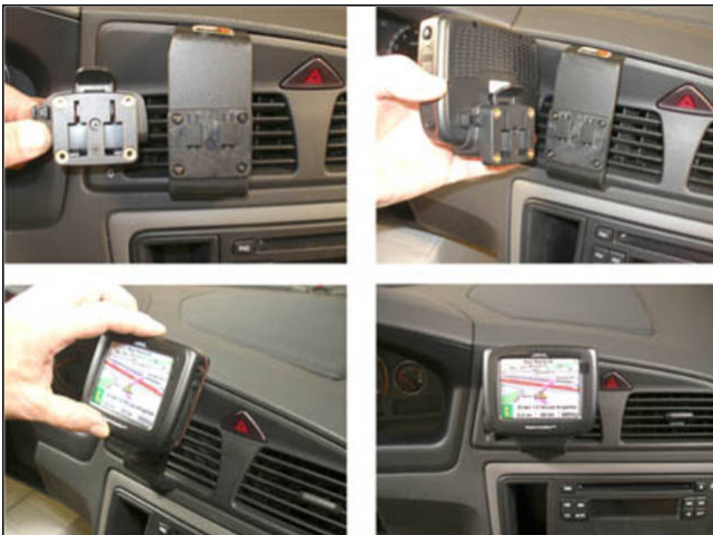
3. Now that the plate is in place, find your device cradle, which is usually enclosed with your device when purchased. (Magellan 2000 shown in picture). Attach your device cradle to your device, then hook the device with the cradle onto the T prongs and slide it down. If you don't have a cradle, hook your device onto the T prongs and slide it down. To remove it, slide the device up and unhook it from the T prongs.
