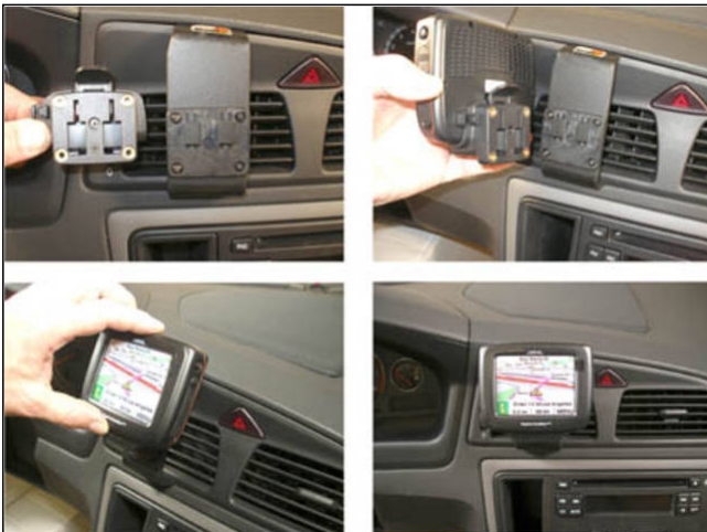
3. Now that the plate is in place, find your device cradle, which is usually enclosed with your device when purchased. (Magellan 2000 shown in picture). Attach your device cradle to your device, then hook the device with the cradle onto the T prong and slide it down. If you don't have a cradle, hook your device onto the T prong and slide the device up and unhook it from the T prong.
