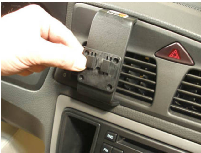
1. Place the 2 prong (Single T) vehicle mounting plate in the desired position.
