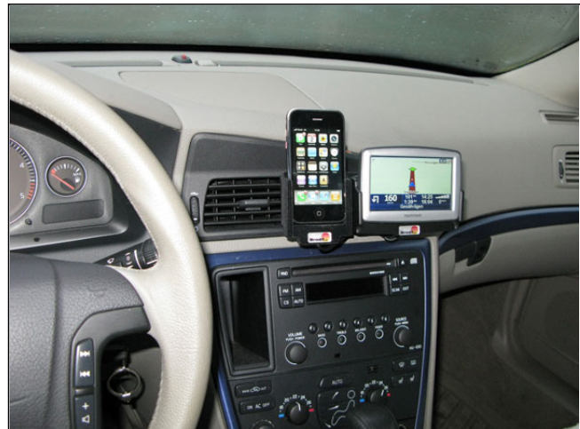
4. The Extension Plate with holders and devices in place. The Devices shown in the picture are an Apple iPhone 3G and a TomTom XL navigation unit.
