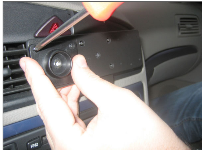
2. Attached the base plate from the Holders tilt swivel to the Extension Plate with the enclosed screws in the Holder packaging.
