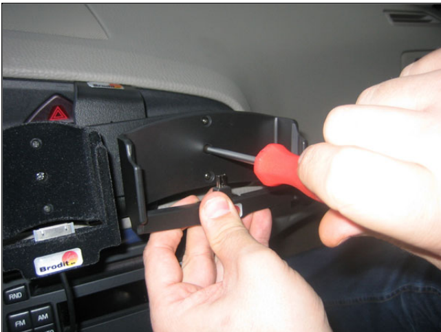
3. Attach your Holder onto the Extension Plate. (see separate instruction enclosed with the Holder)
