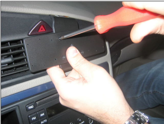
1. Press a screwdriver (Philips) firmly through the pre-drilled holes in the Extension Plate to open them up. Place the Extension Plate over the matching holes in your mounting bracket. Attach it by using the applicable screws enclosed - self-tapping screws if the mount has small holes or machine screws with nuts if the mount has large holes.
