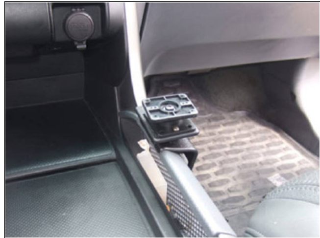
2. Attaching the Angled Extension Plate directly onto a ProClip Vehicle Mount with a Tilt Swivel: Attach the Tilt Swivel Mount to the ProClip Vehicle Mount. The Tilt Swivel Mount allows for better adjustment and viewing.
