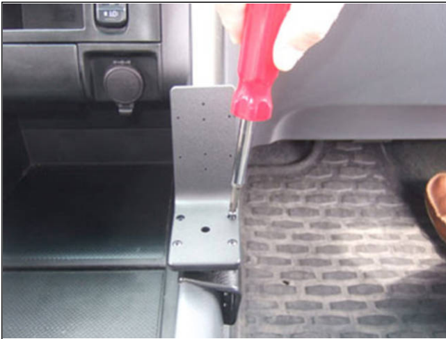
1. Attaching the Angled Extension Plate directly onto a ProClip Vehicle Mount: Place the Angled Extension Plate over the matching holes in the Vehicle Mount and attach it with the 4 applicable screws.
