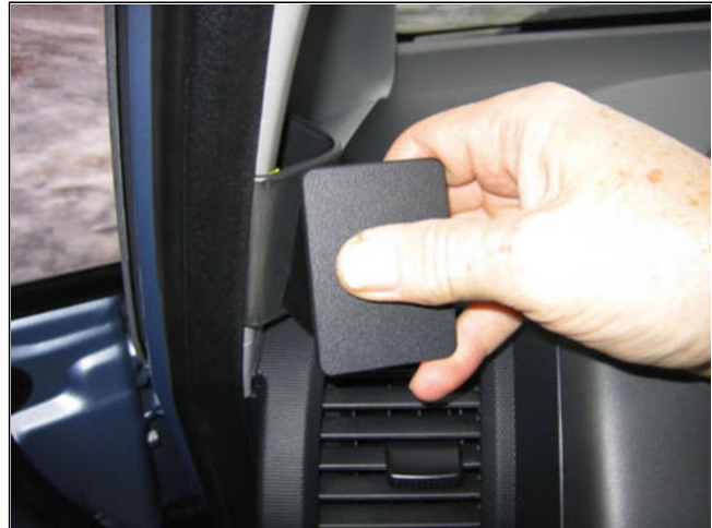
2. Press forwards on the right side of the ProClip so the long right end hooks behind the edge by the window.
