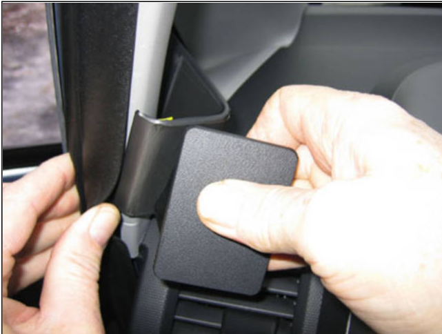
1. Peel off the adhesive tape covers on the ProClip. Pull out the rubber covering and hook the angled left edge of the ProClip behind the edge.
