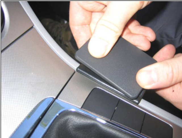
1. Peel off the adhesive tape covers on the ProClip. Press the angled edge on the left side of the ProClip into the gap between the panel surrounding the gear shift and the edge of the console.
