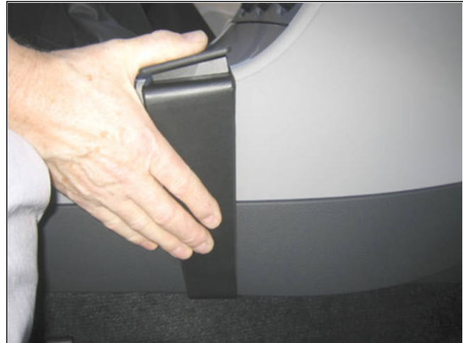
2. Press downwards on the right side of the ProClip so the angled edge hooks under the edge of the console.
