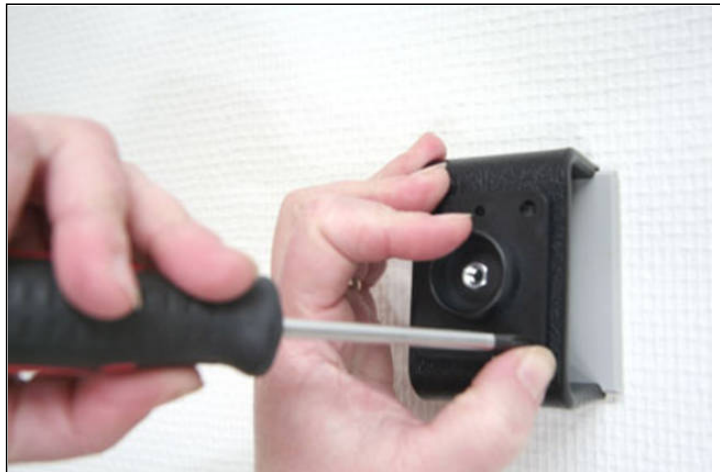
2. Place the base plate over the matching holes in your mounting bracket (demo ProClip mount shown in picture) Attach the base plate by using the self-tapping screws. Note: The machine screws with nuts are for mounts made of metal with large holes.
