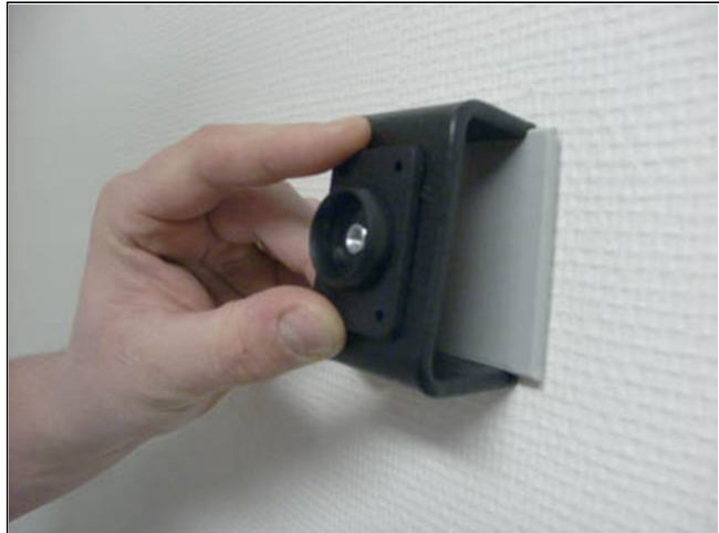
2. Place the base plate over the matching holes in your mounting bracket (demo ProClip mount shown in picture) Attach the base plate by using the self-tapping screws. Note: The machine screws with nuts are for mounts made of metal with large holes.
