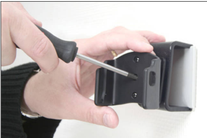
3. Start to thread the center screw into the base plate. When you connect with the nut pull the holder towards you to prevent the nut from spinning around. Continue to tighten the screw firmly. Then loosen the screw slightly for easier angling/rotation of the holder.
