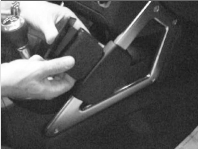
1. Clean the surface with the enclosed alcohol pad. Peel off the adhesive tape cover on the ProClip.
