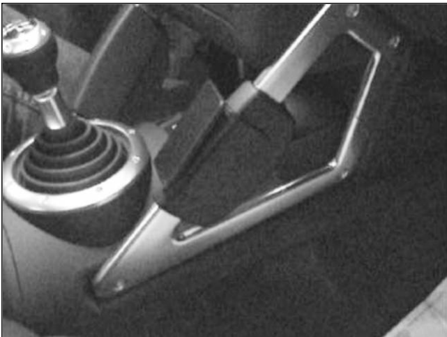
3. Press down on top of the ProClip towards the floor until the angled edge on the left side of the Proclip under the padded edge.
