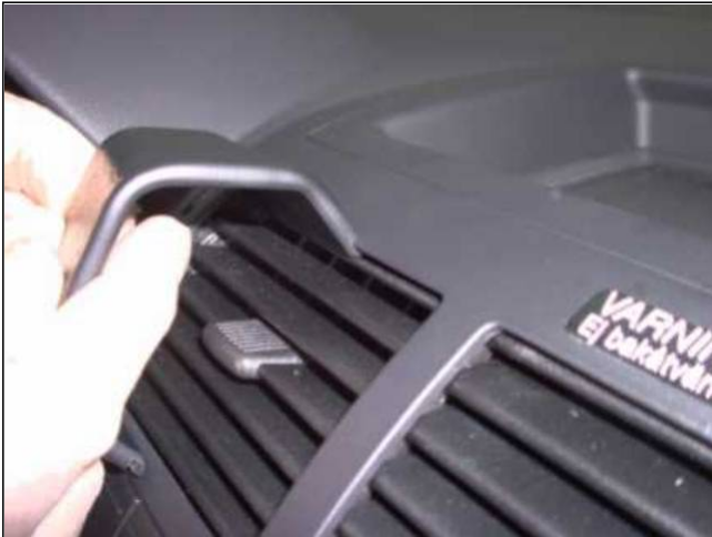
1. Hook the upper part of the ProClip, with groove, behind the upper edge of the air vent housing.
