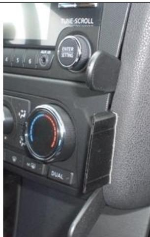
3. Press the angled edges firmly into the gap and at the same time rotate Part 1 to the right until you see or hear/feel it clip into place behind the panel. Don't press the tape towards the console edge yet. First, slide Part 1 downwards until it stops. Then press Part 1 towards the console edge so the adhesive tape attaches. Pull out the gap openers.
