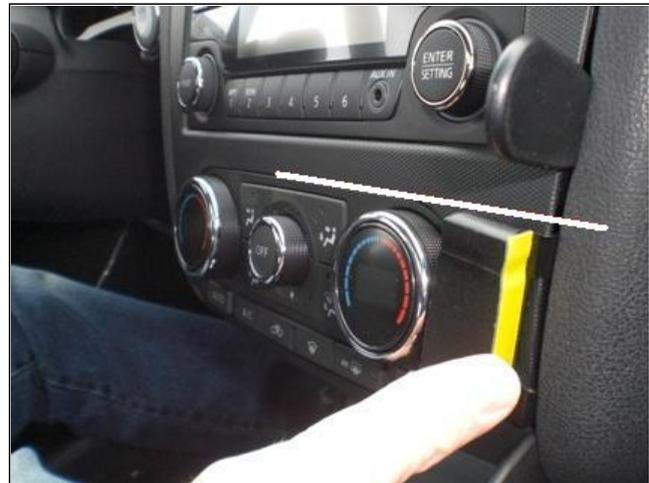
2. Align the top of Part 1 with the panel line above the temperature controls to the left of the opened gap (notice the bold line in the photo) Or measure 5 1/8 down from the top of the seam.
