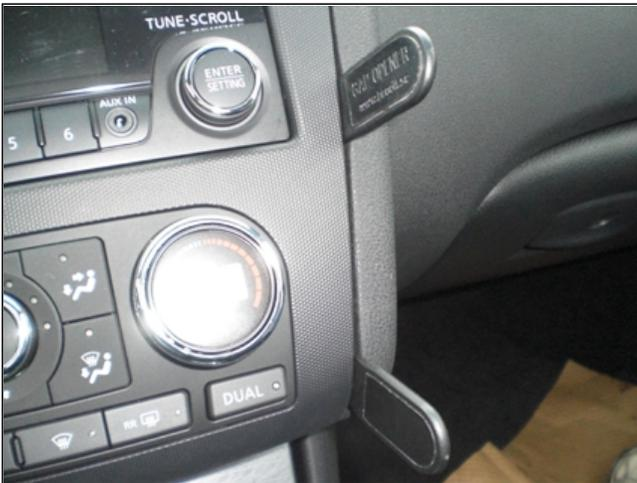
1. Attention! This ProClip consists of two parts. Part 1 - ProClip attaching part (the smallest part) and Part 2 is the ProClip face plate. Press the thin end of one enclosed gap opener into the gap between the center console panel frame and the padded part of the dashboard. Press the second gap opener into the gap at the lower corner. Push both gap openers in until they stop, to widen the gap. Peel off the cover of the adhesive tape on Part 1.
