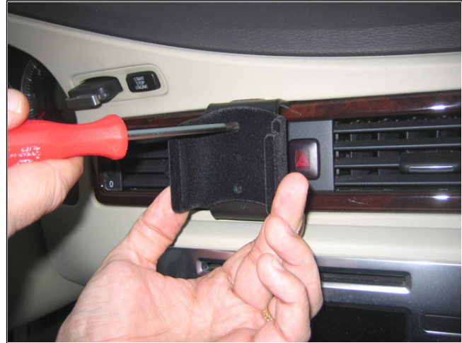
2. Attach the holder by using the self-tapping screws. Note: the machine screws with nuts are for mounts made of metal with large holes.
