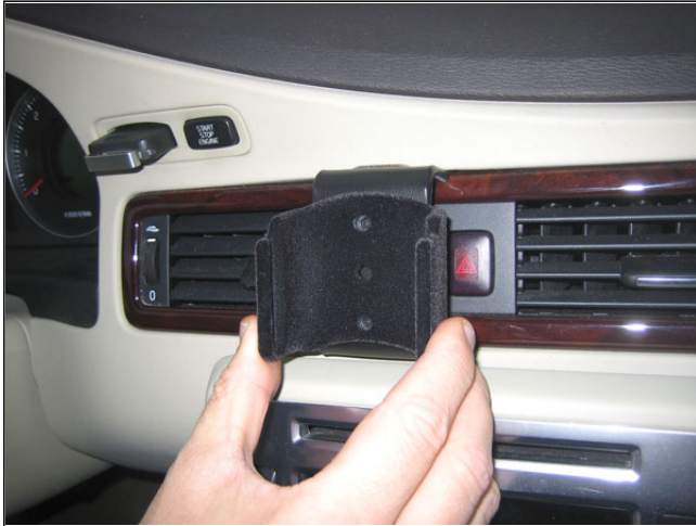
1. Place the holder over the matching holes in your mounting bracket. (ProClip Vehicle Mount shown in picture)
